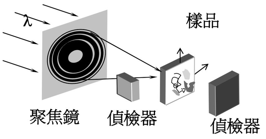
STXM(Scanning Transmission X-ray Microscopy)
